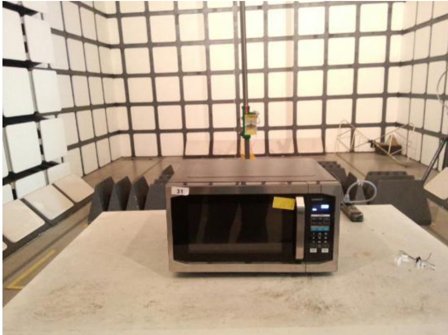
Operating Frequency Test Set-up
