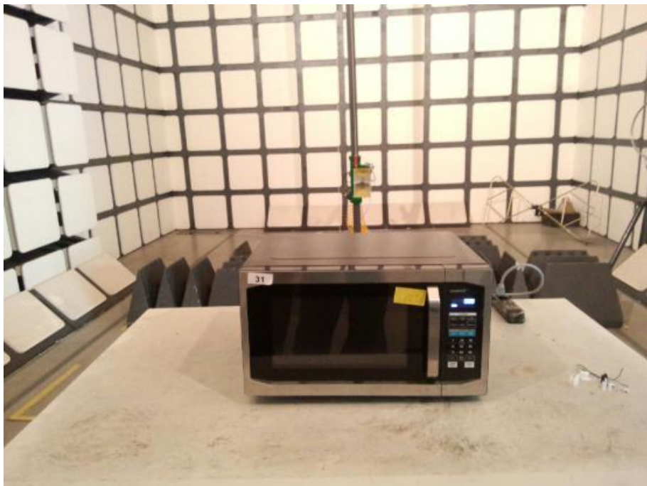
Radiated Emission Test Set-up (1-18GHz)
