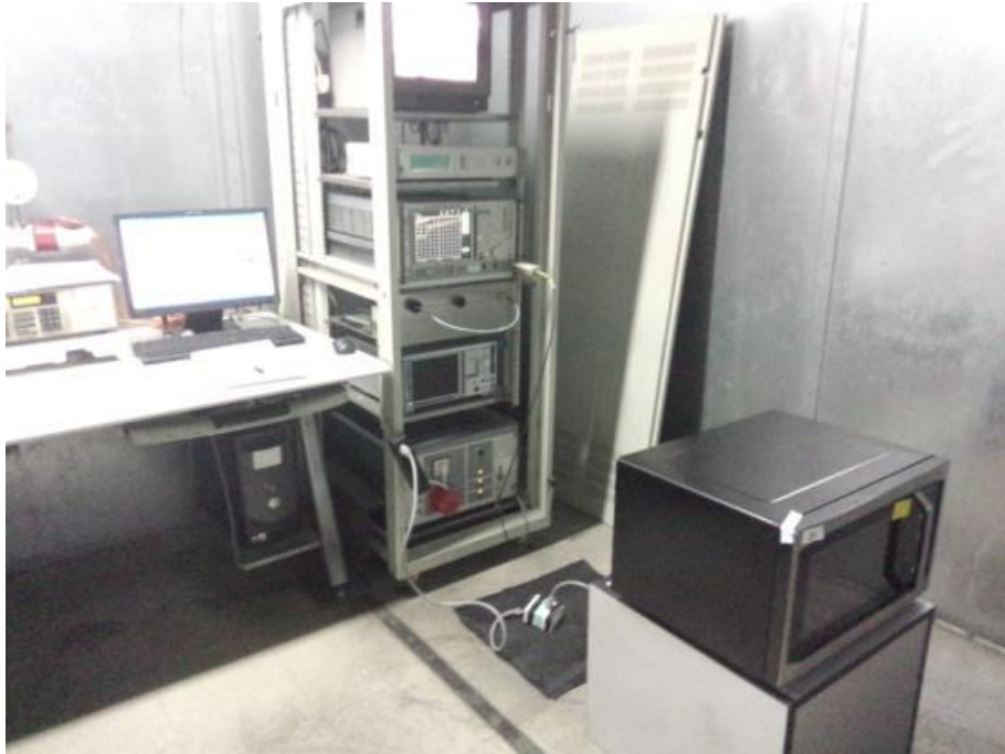
Conducted Emission Test Set-up
