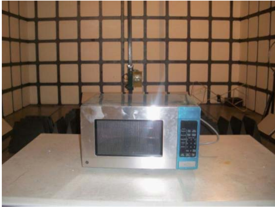
Radiated Emission Test Set-up (1-18GHz)
