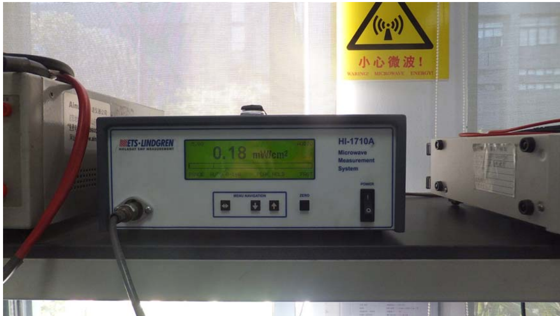
Radiation Hazard Test Set-up
