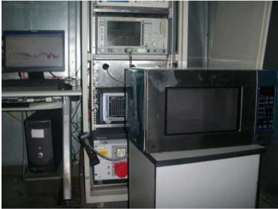
Conducted Emission Test Set-up
