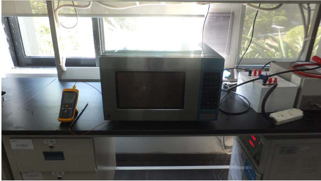
RF Output Power Test Set-Up
