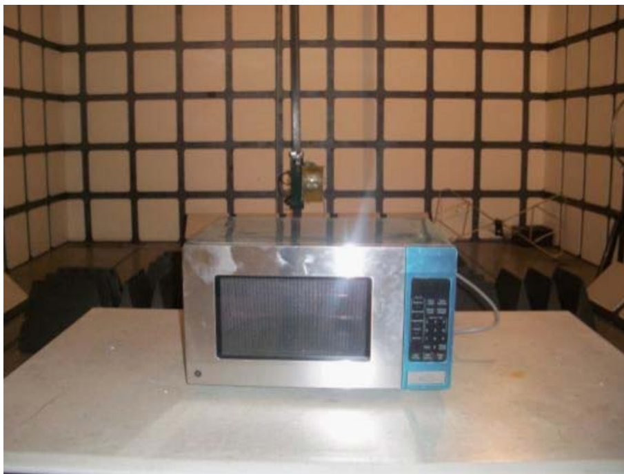
Operating Frequency Test Set-up
