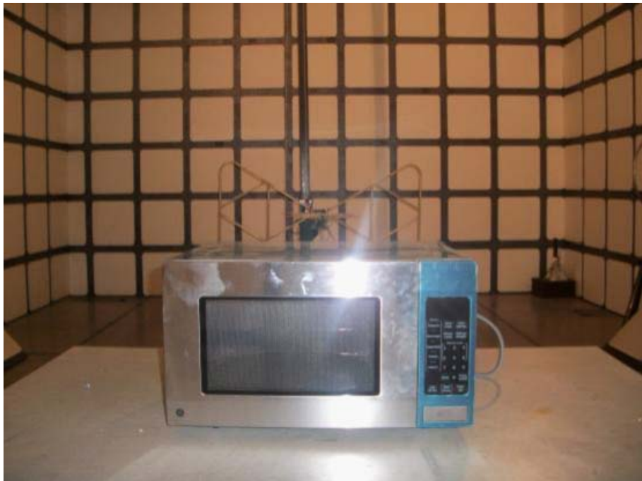
Radiated Emission Test Set-up (30 -1,000MHz)
