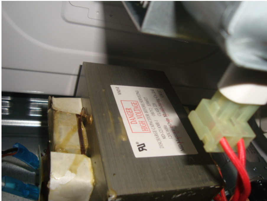
High Voltage Transformer View
