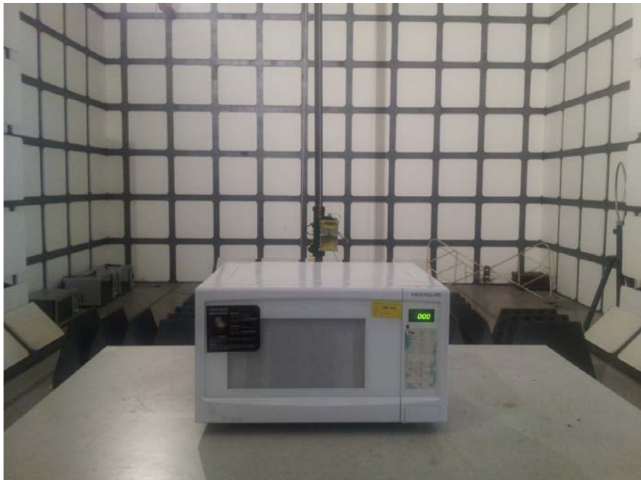
Operating Frequency Test Set-up
