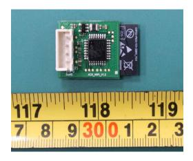
The New Connection PCB of Wi-Fi module.
