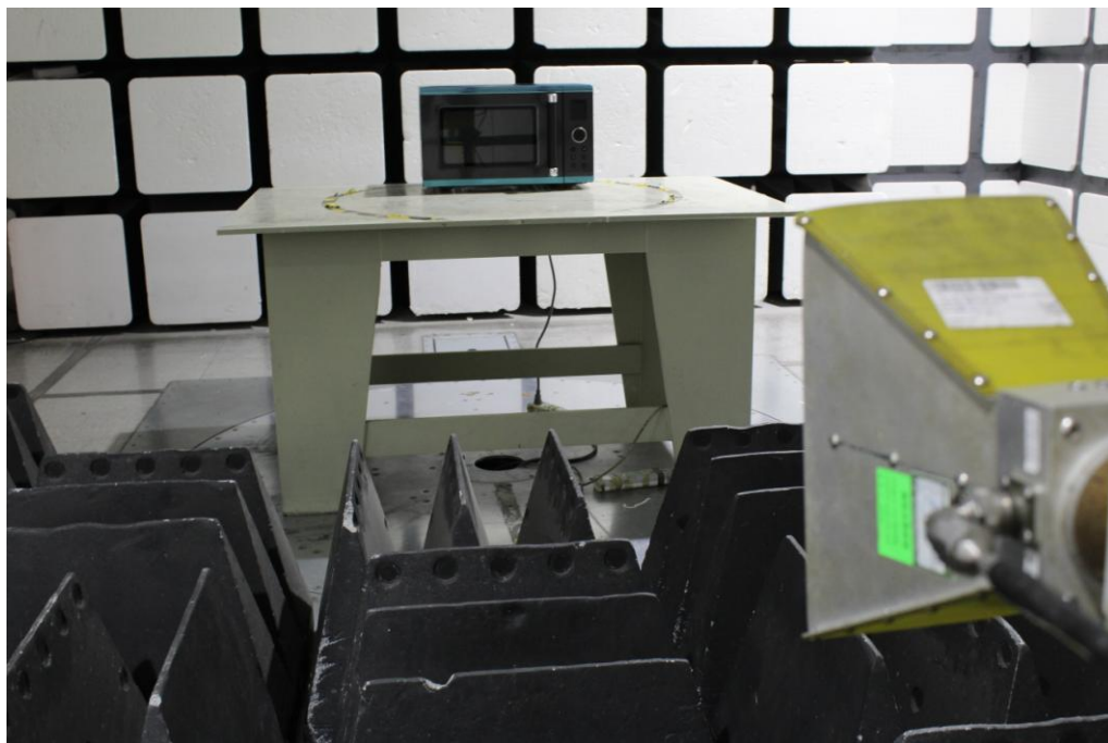
Radiated Emissions - Front View (Above 1 GHz)
