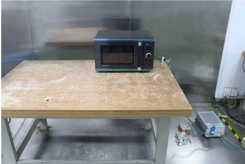
Conducted Emissions - Side View
