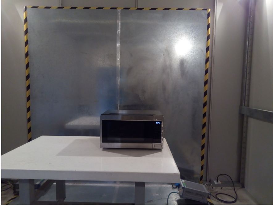
Conducted Emissions - Front View
