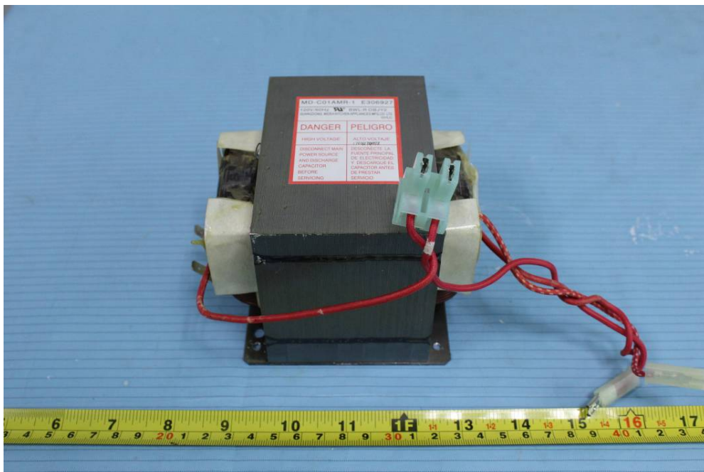
EUT –Transformer View
