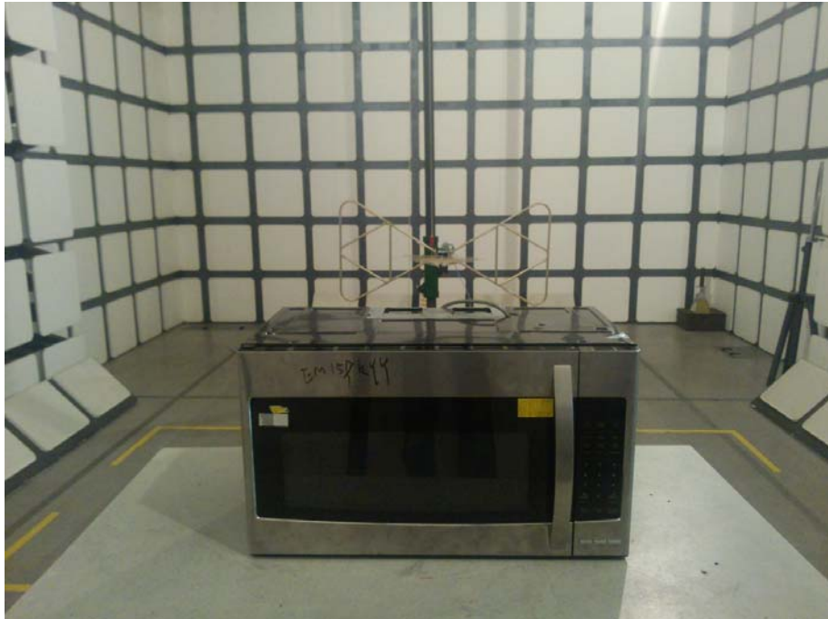
Radiated Emission Test Set-up (30 - 1,000MHz)
