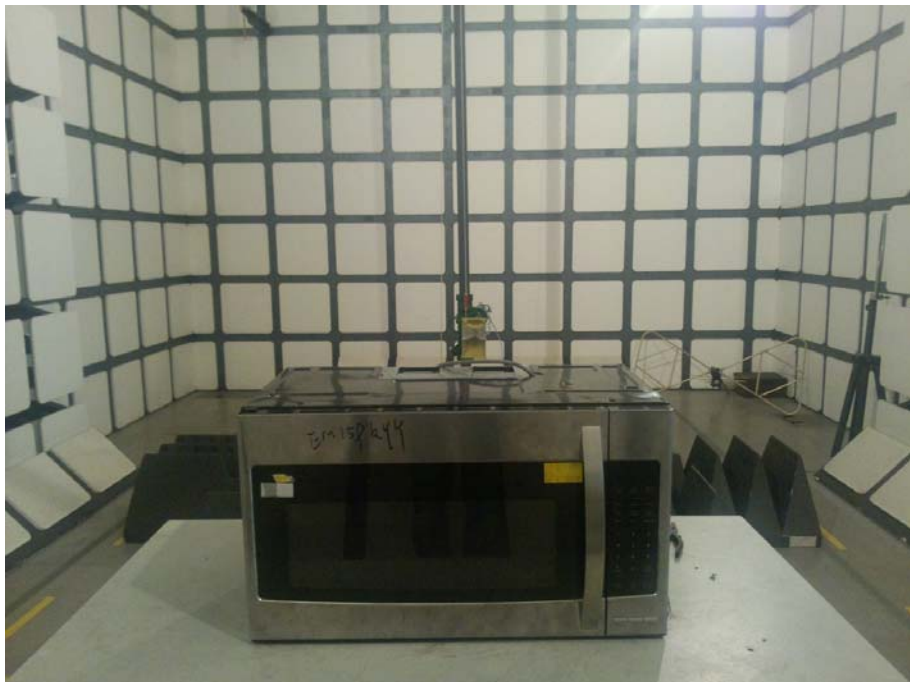
Radiated Emission Test Set-up (1-25GHz)
