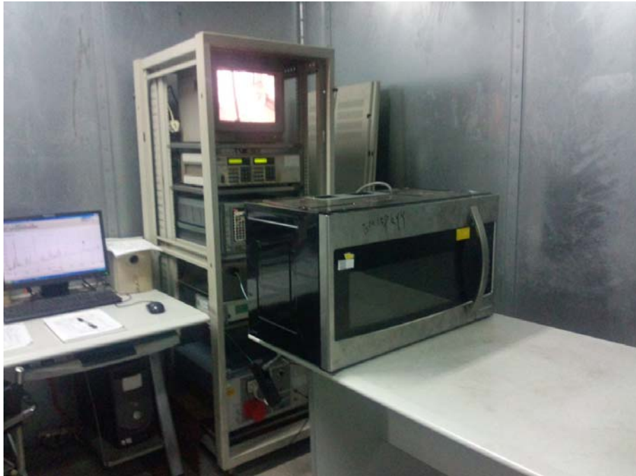
Conducted Emission Test Set-up
