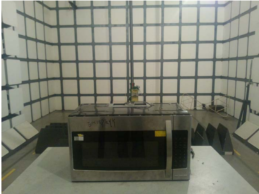
Operating Frequency Test Set-up
