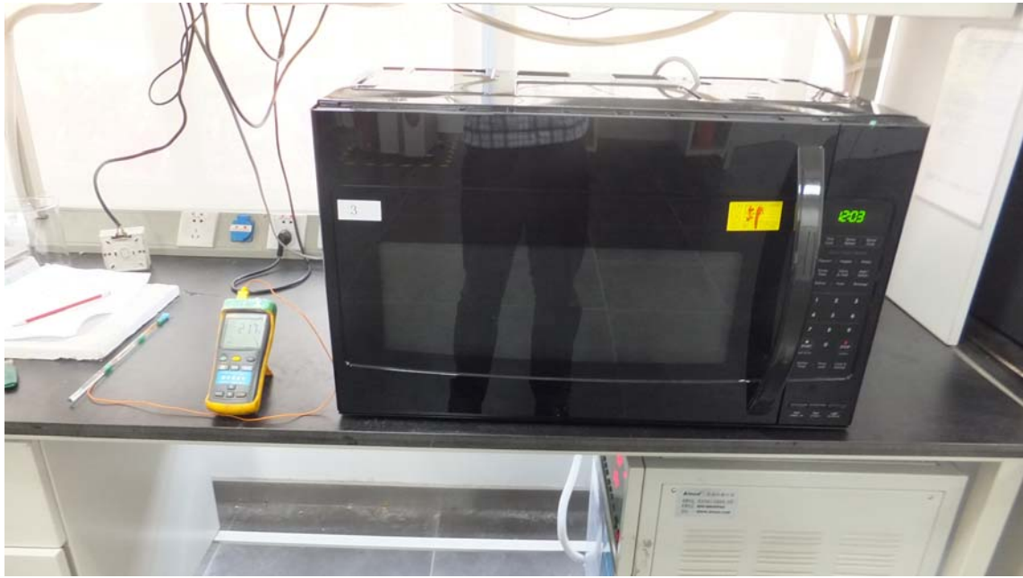
RF Output Power Test Set-Up
