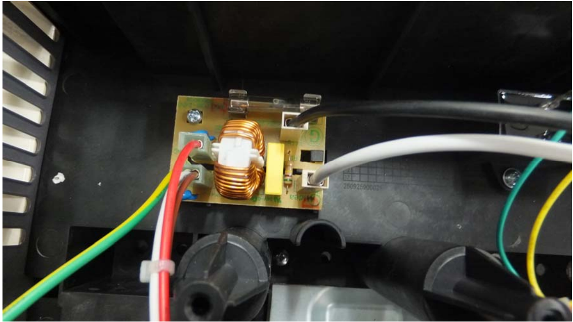
Power Filter Board Top View
