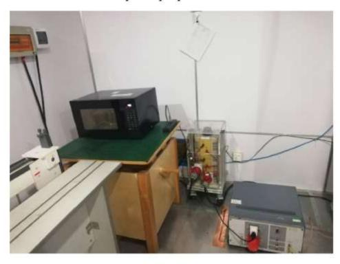
Radiated Emission Measurement below 1GHz
