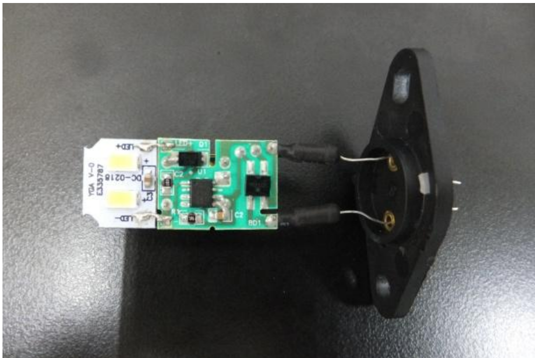
LED Lamp 2: PCB board- Bottom View
