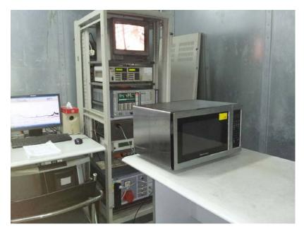
Radiated Emission Test Set-up (30 -1,000MHz):
