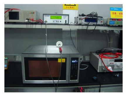
**Input Power Test Set-Up :**
