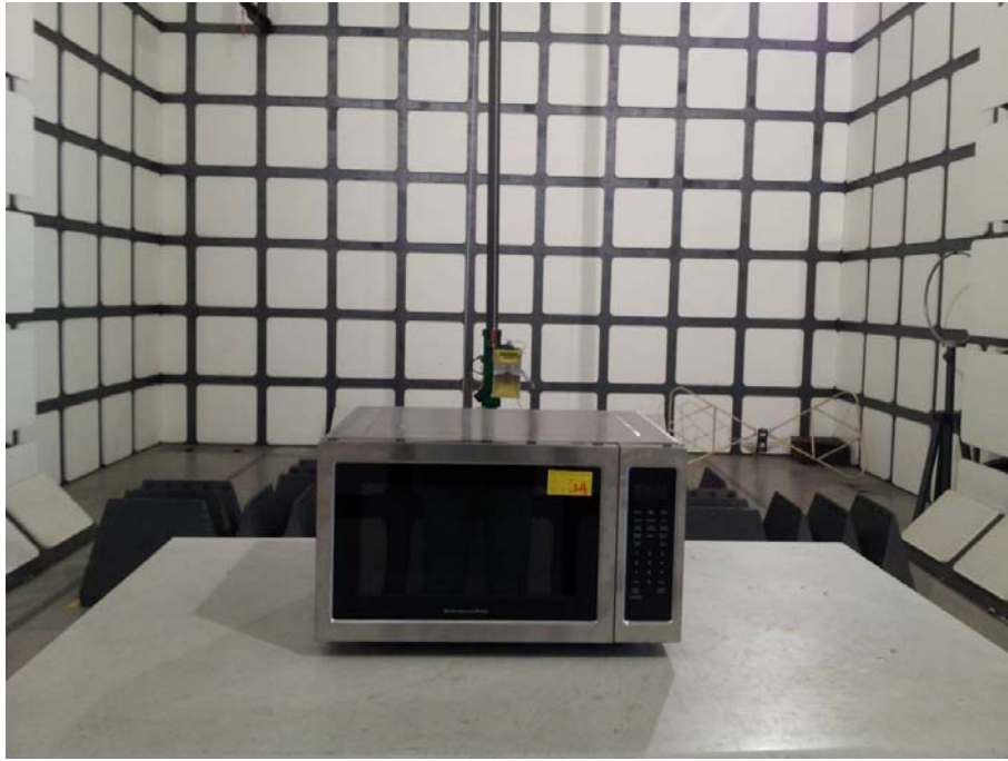
Operating Frequency Test Set-up
