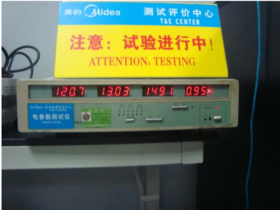
Input Power Test Set-Up
