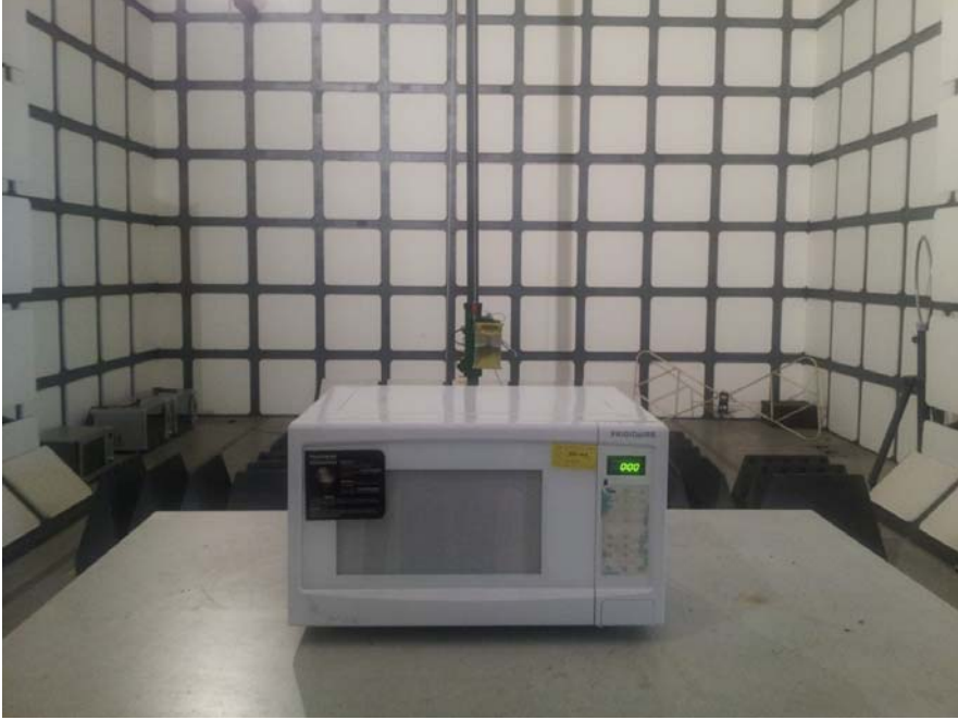
Operating Frequency Test Set-up
