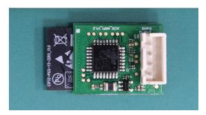
The New Connection PCB of Wi-Fi module.
