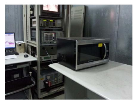
Radiated Emission Test Set-up (30 -1,000MHz):
