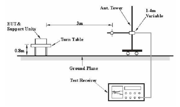
The radiated emission tests were performed in the 3 meters chamber A test site, using the setup accordance with the FCC MP - 5. The specification used was the FCC part 18 limits.
