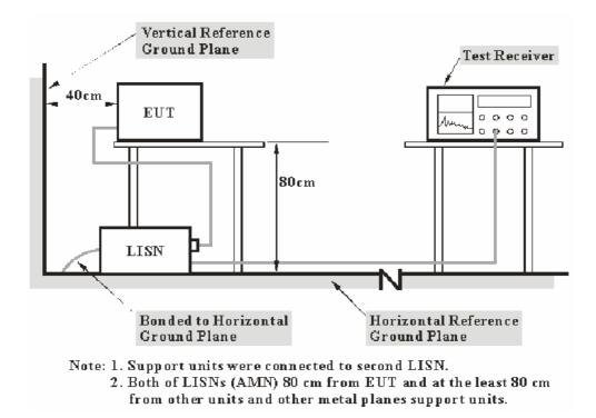
The setup of EUT is according with per MP-5: 1986 measurement procedure. Specification used was with the FCC Part 18.
