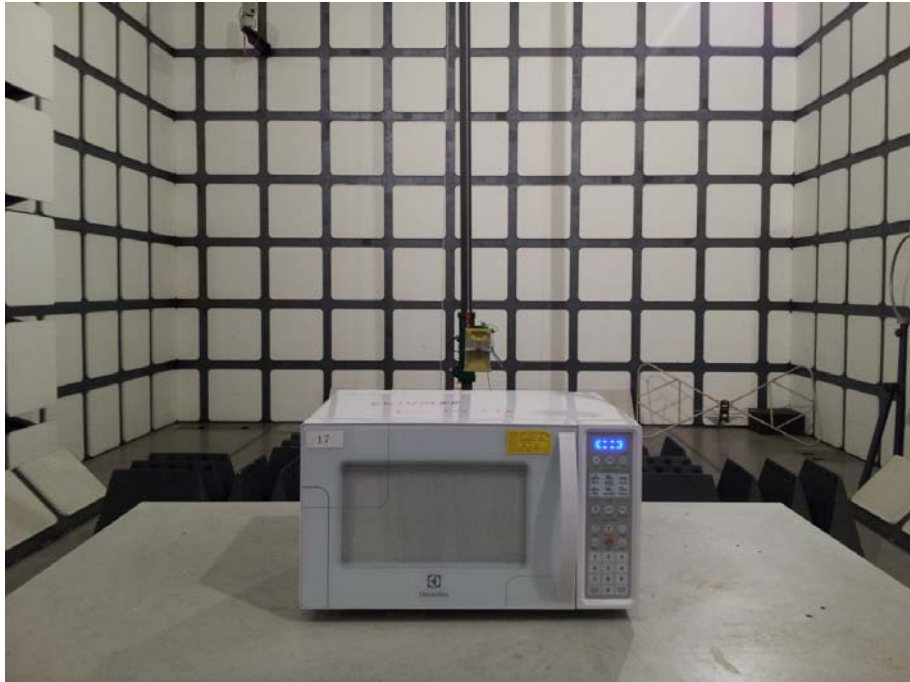
Operating Frequency Test Set-up
