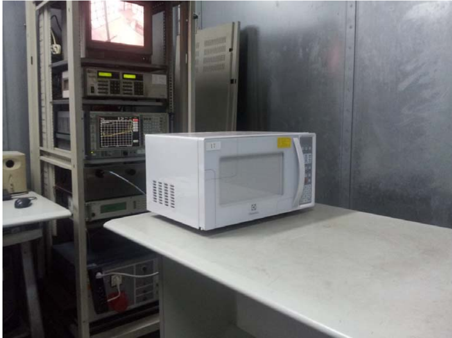
Conducted Emission Test Set-up
