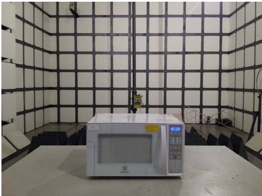
Radiated Emission Test Set-up (1-18GHz)
