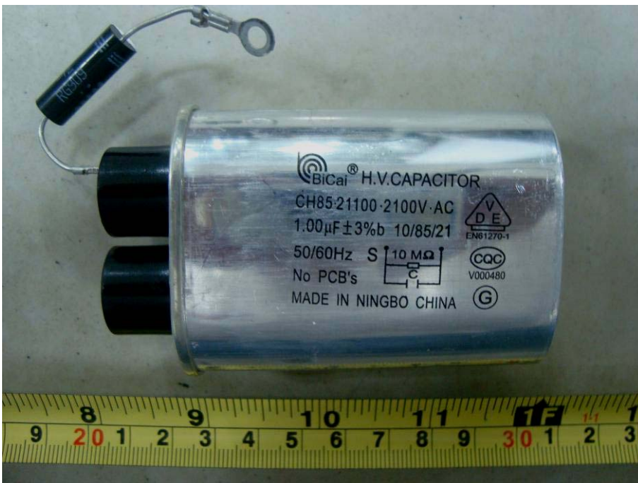
EUT – Capacitor View
