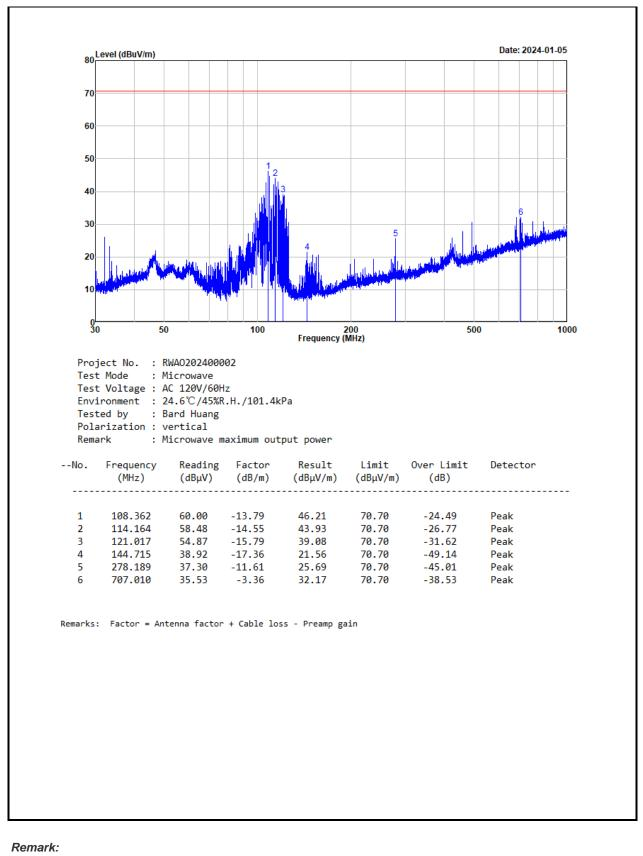
Result = Reading + Factor Factor = Antenna factor + Cable loss – Amplifier gain Over Limit = Result – Limit
