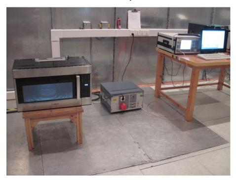
Radiated Emission Test Set-up (30 -1,000MHz):
