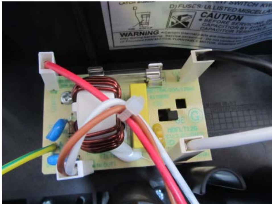
Power Filter Board Top View
