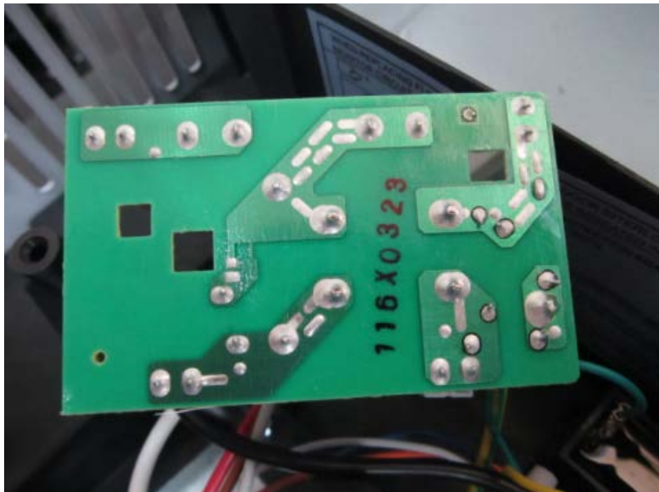
Power Filter Board Bottom View
