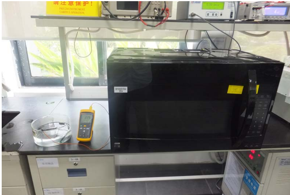
RF Output Power Test Set-Up
