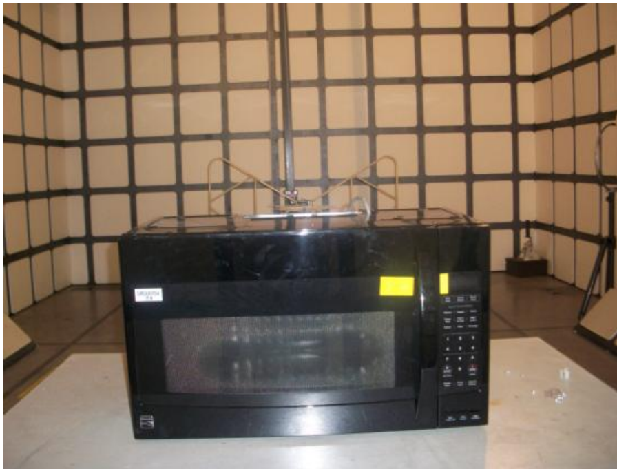
Radiated Emission Test Set-up (30 - 1,000MHz)
