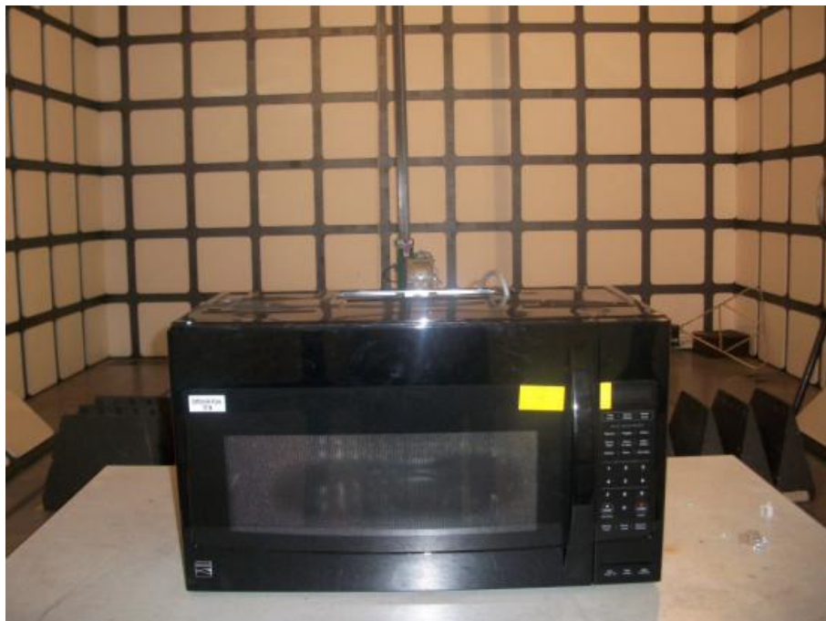
Operating Frequency Test Set-up
