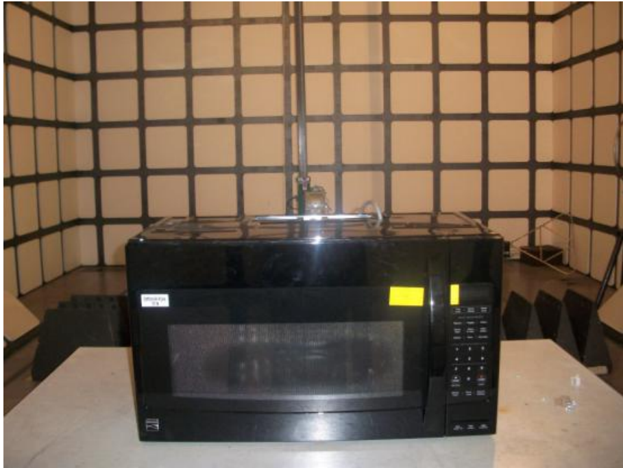
Radiated Emission Test Set-up (1-18GHz)
