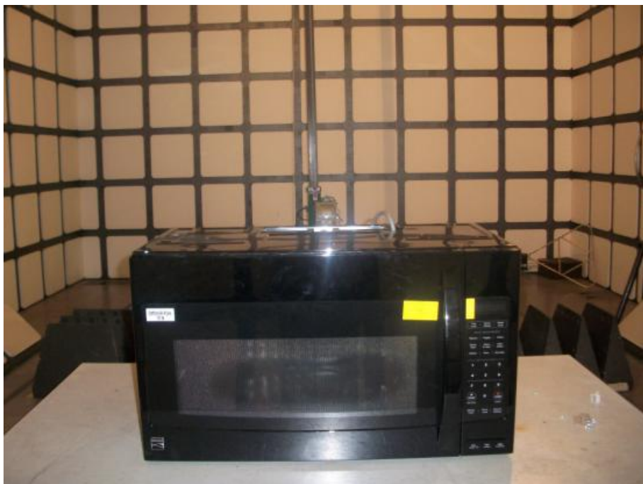
Radiated Emission Test Set-up (1-18GHz)
