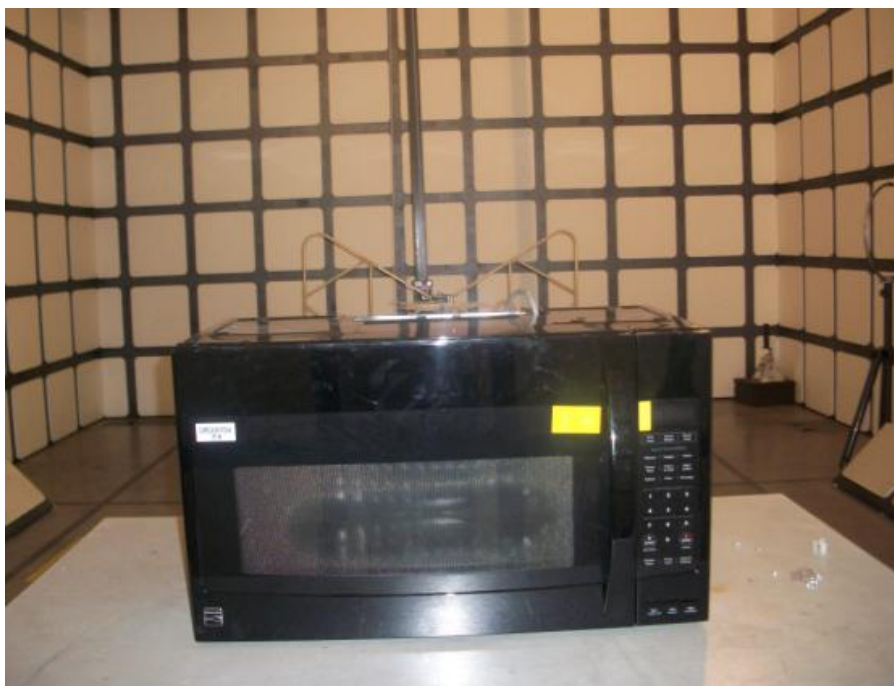
Radiated Emission Test Set-up (30 -1,000MHz)
