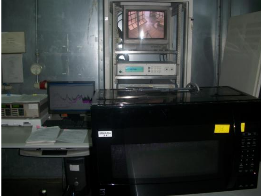
Conducted Emission Test Set-up
