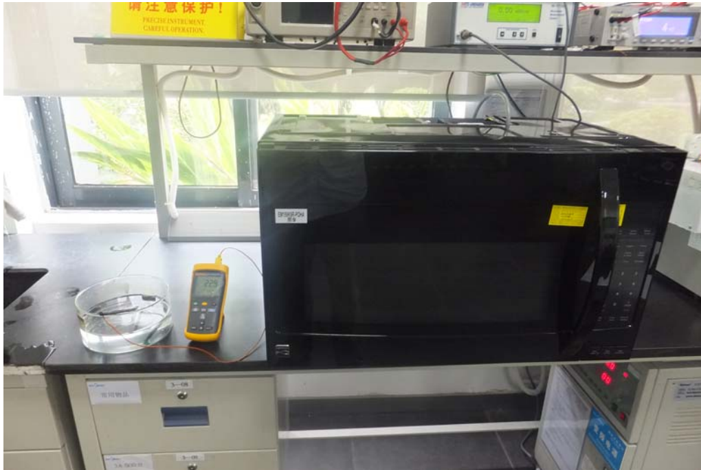
RF Output Power Test Set-Up
