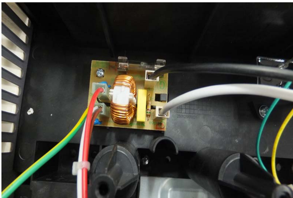
Power Filter Board Top View
