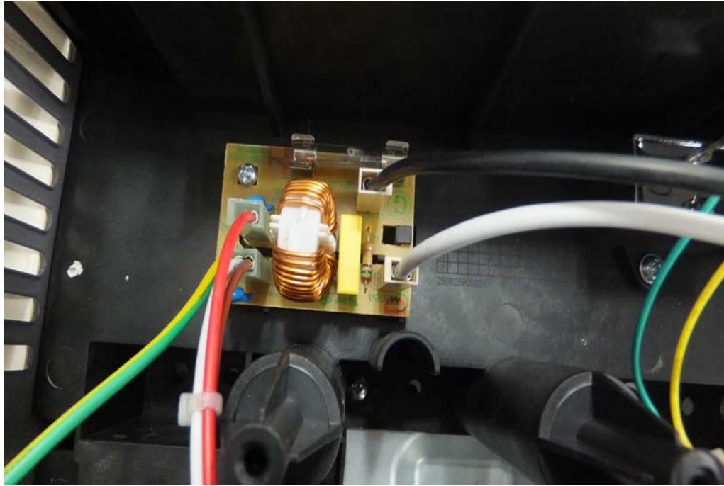
Power Filter Board Top View
