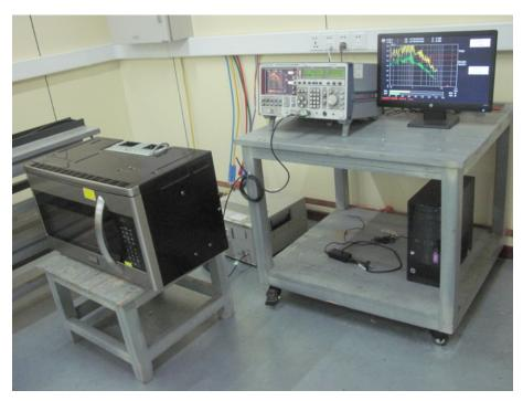
Radiated Emission Test Set-up (30 -1,000MHz):
