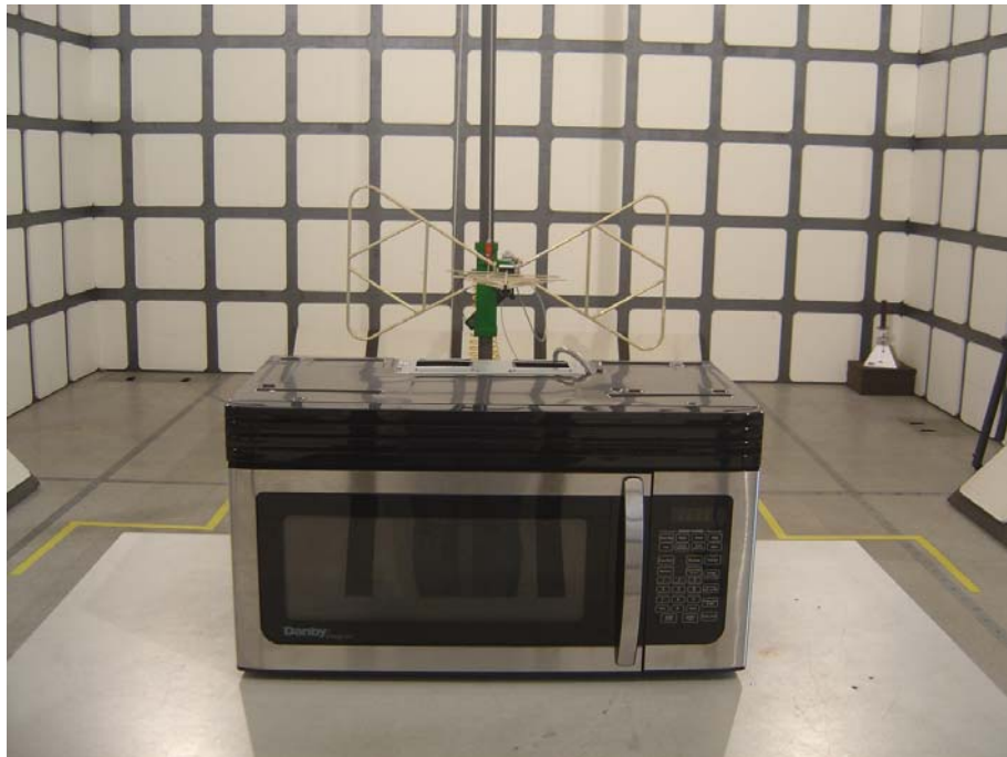
Radiated Emission Test Set-up (30~1000MHz):
