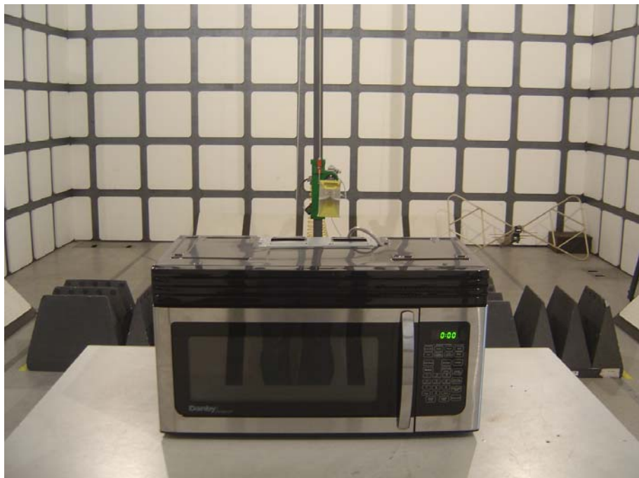
Radiated Emission Test Set-up (1~25GHz):
