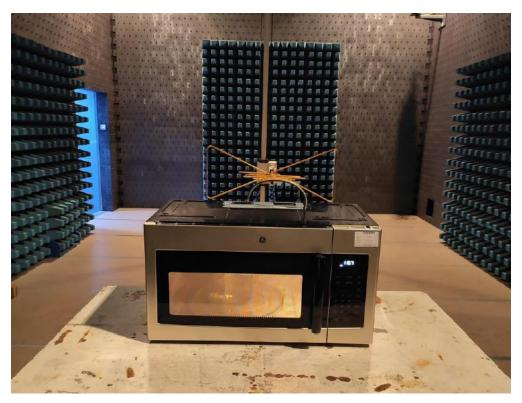
Radiated Emission Test Set-up (1-25GHz):
