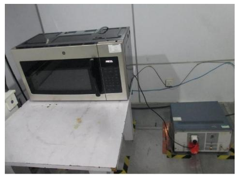
Radiated Emission Test Set-up (30 -1,000MHz):
