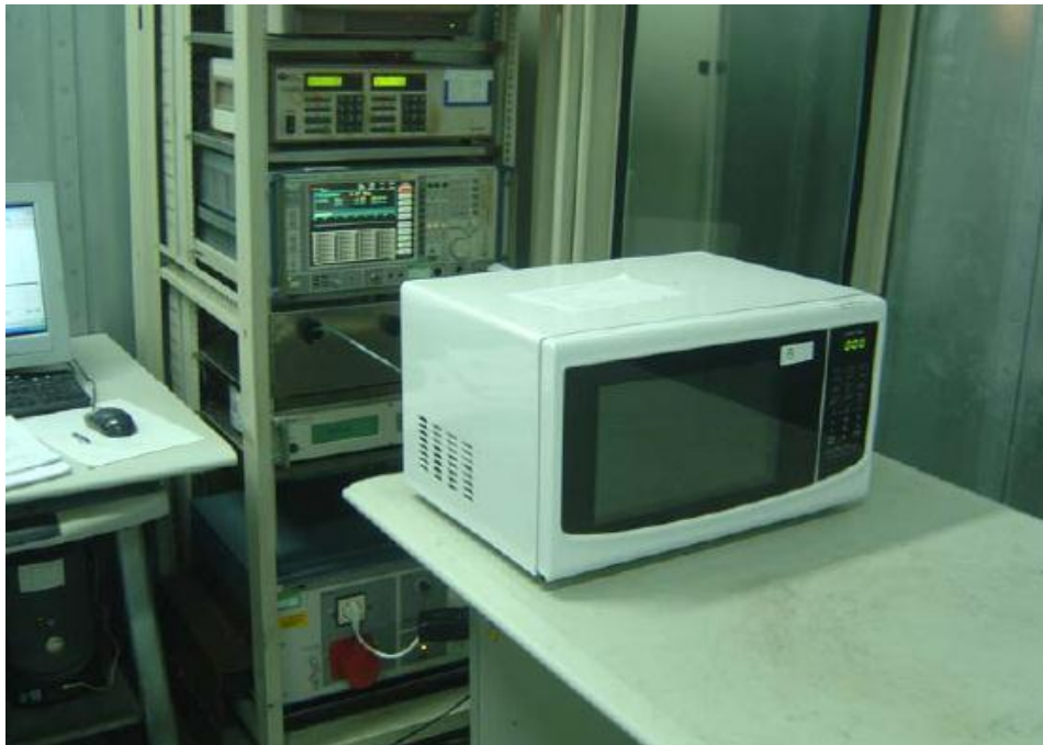
Conducted Emission Test Set-up
