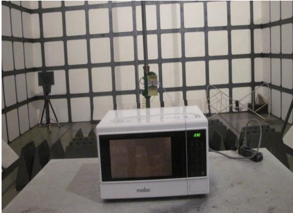
Operating Frequency Test Set-up
