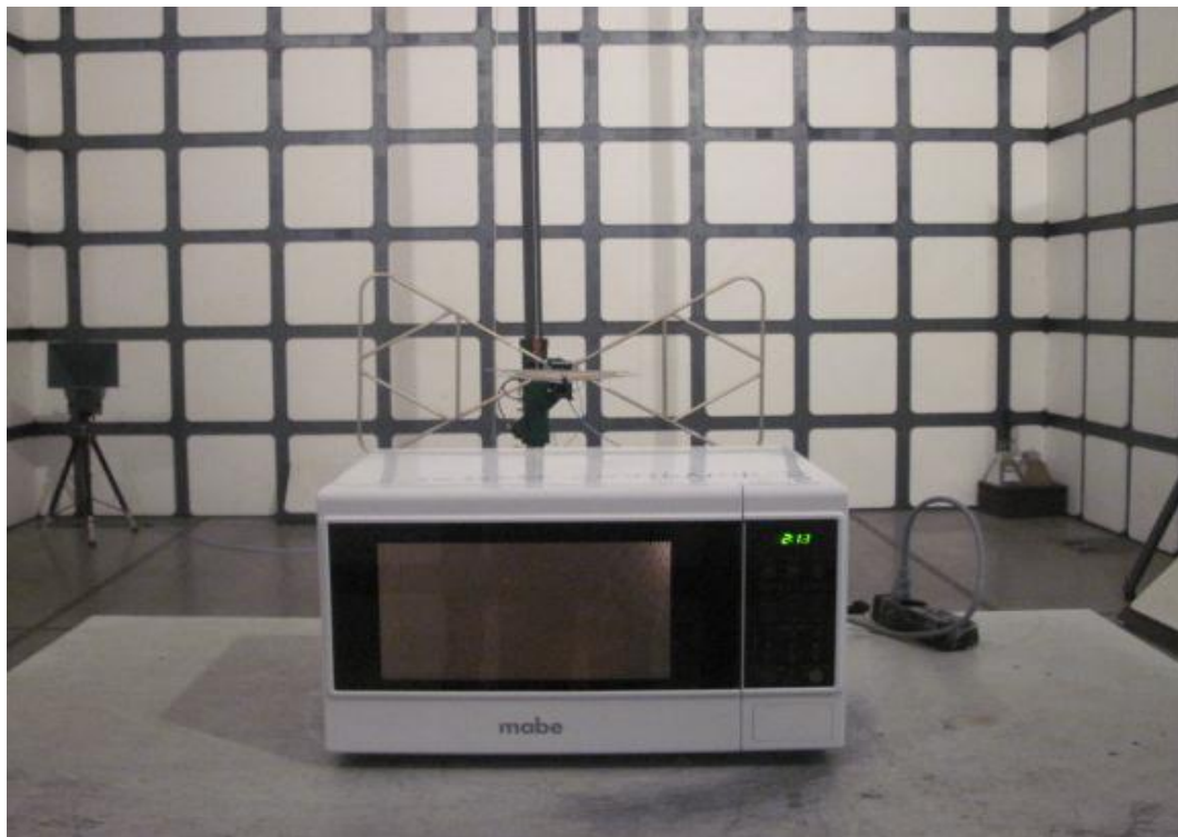
Radiated Emission Test Set-up (30 -1,000MHz)
