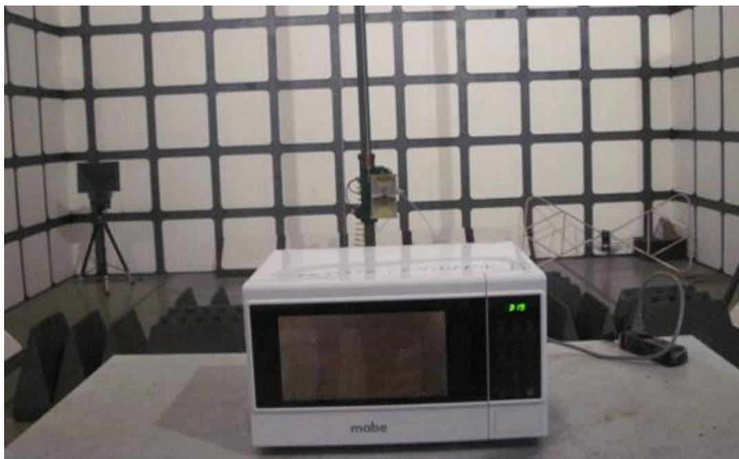
Radiated Emission Test Set-up (1-25GHz)
