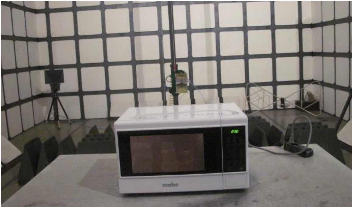
Operating Frequency Test Set-up
