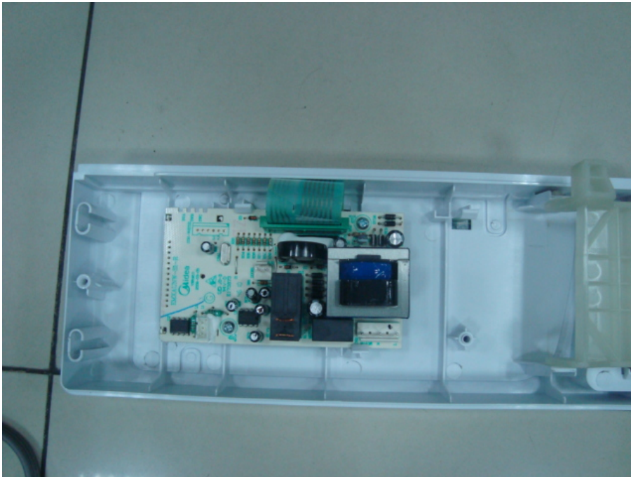
Control Board Rear View
