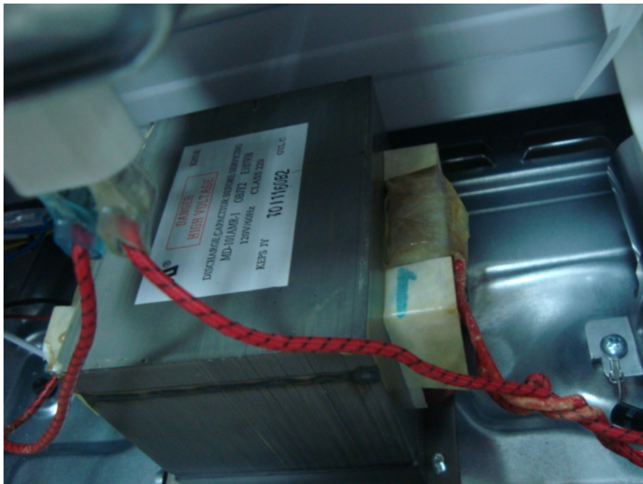
High-voltage Transformer View
