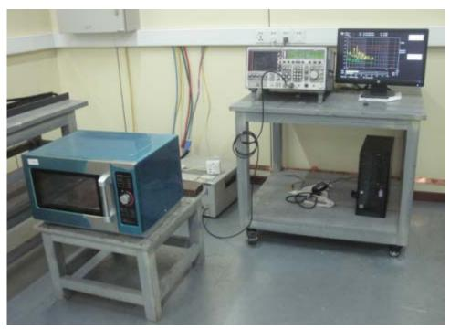
Radiated Emission Test Set-up (30 -1,000MHz):
