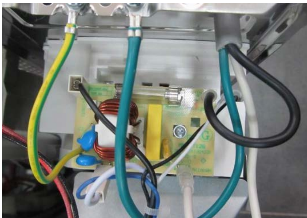
Power Filter Board Top View
