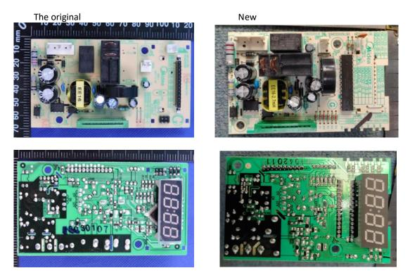
They have the same input and output rating(s) except for PCB layout and some components.
