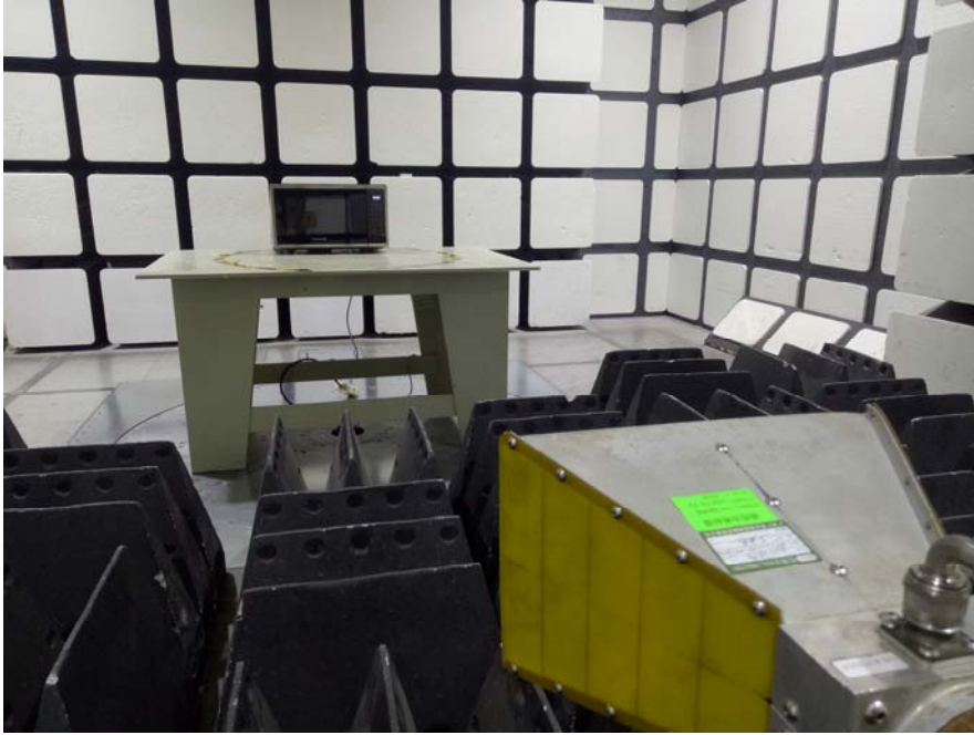
Radiated Emissions - Front View (Above 1 GHz)
