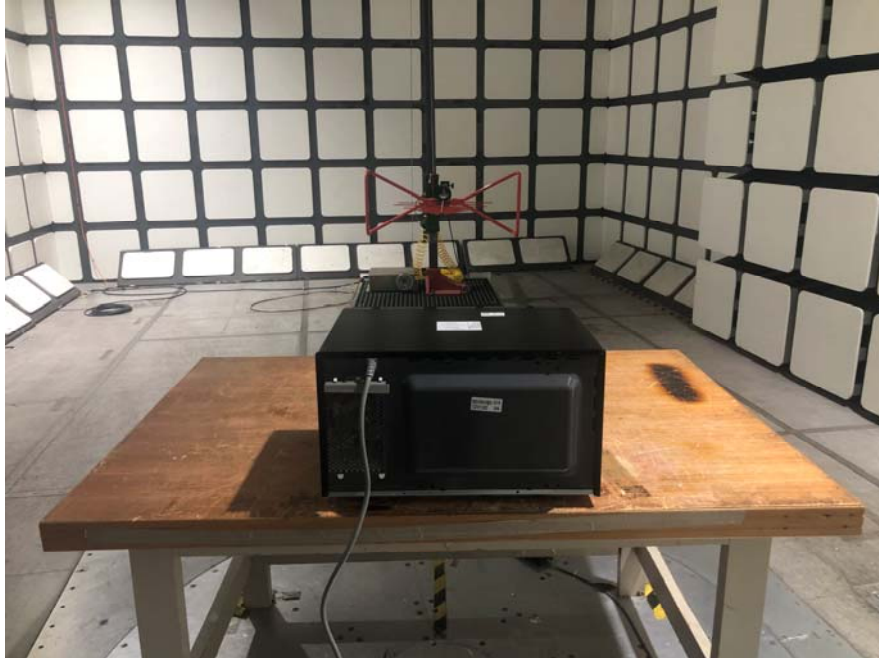
Radiated Emissions - Rear View (30 MHz – 1 GHz)
