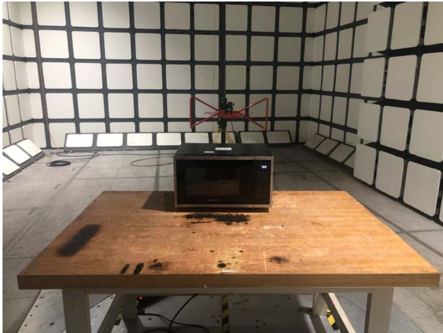
Radiated Emissions - Front View (30 MHz – 1 GHz)
