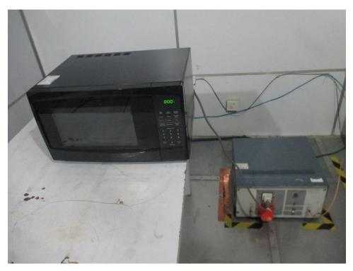
Radiated Emission Test Set-up (30 -1,000MHz):
