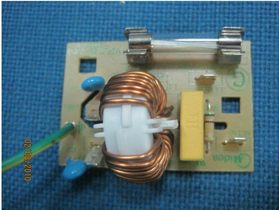
Power Filter Board Top View
