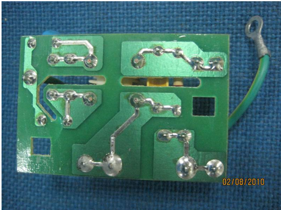
Power Filter Board Bottom View
