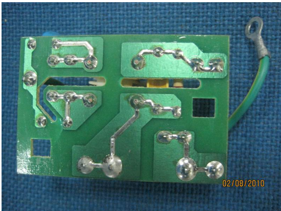
Power Filter Board Bottom View
