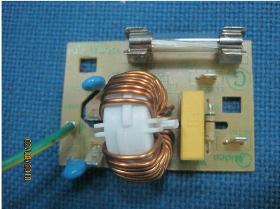
Power Filter Board Top View
