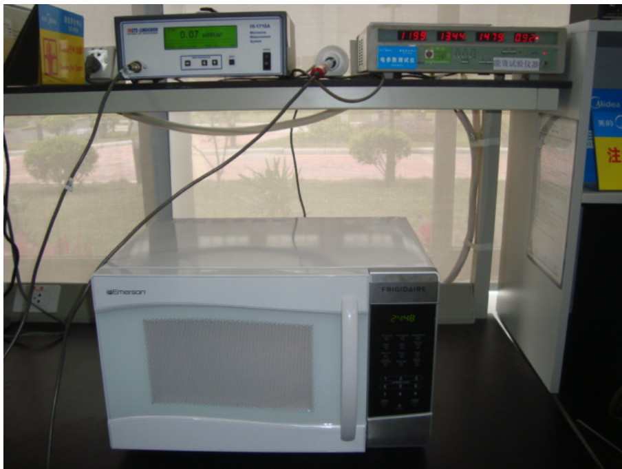
Input Power Test Set-Up :
