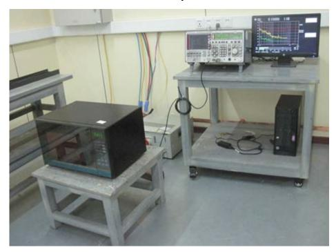
Radiated Emission Test Set-up (30 -1,000MHz):
