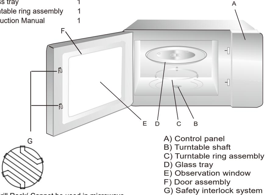
Grill Rack( Cannot be used in microwave function and must be placed on the glass tray )
