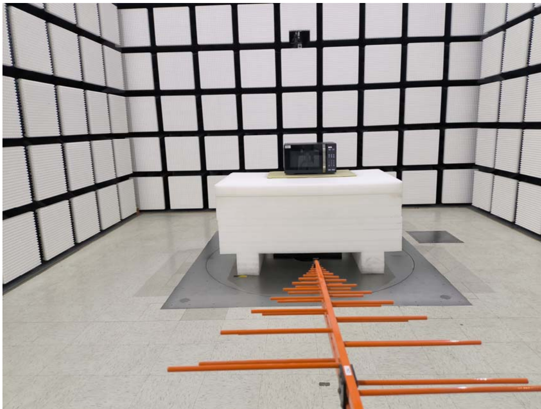
Radiated Emission Below 1GHz Rear View
