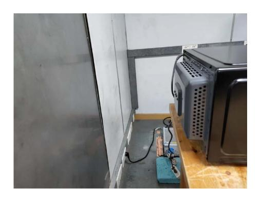
Photo of Radiated Emission Measurement 30 MHz - 1 GHz
