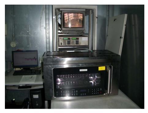
Radiated Emission Test Set-up (30 -1,000MHz)
