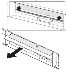
4 Open the light cover (behind the filter mount) by carefully pulling up on its front edge.
