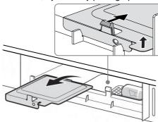
5 Remove the old light bulb and replace with a new, equivalent bulb. Do not use a bulb larger than 30W.
