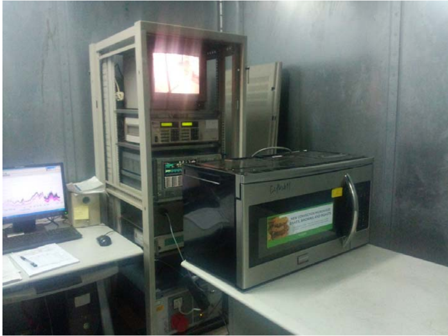
Conducted Emission Test Set-up:
