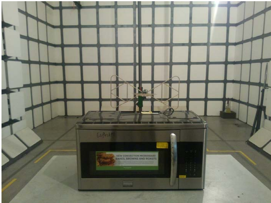
Radiated Emission Test Set-up (30 -1,000MHz):
