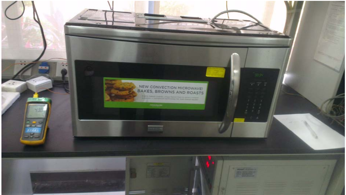
RF Output Power Test Set-Up
