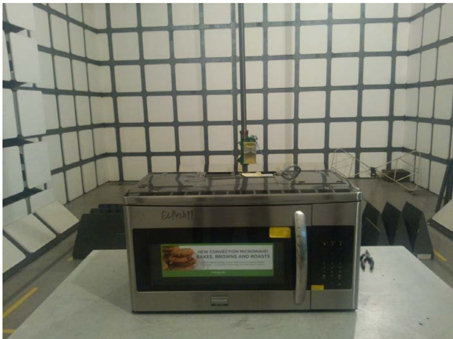
Radiated Emission Test Set-up (1-25GHz)
