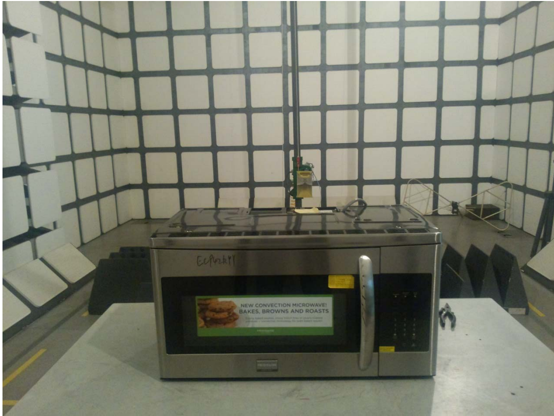
Operating Frequency Test Set-up
