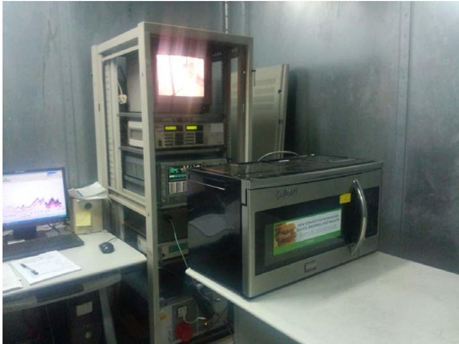
Conducted Emission Test Set-up
