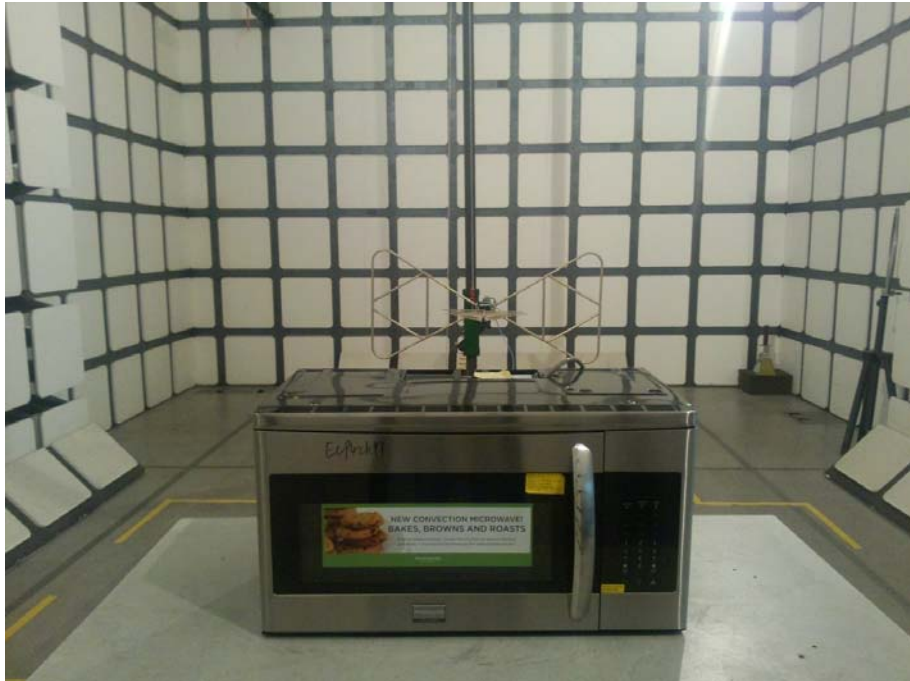
Radiated Emission Test Set-up (30 -1,000MHz)
