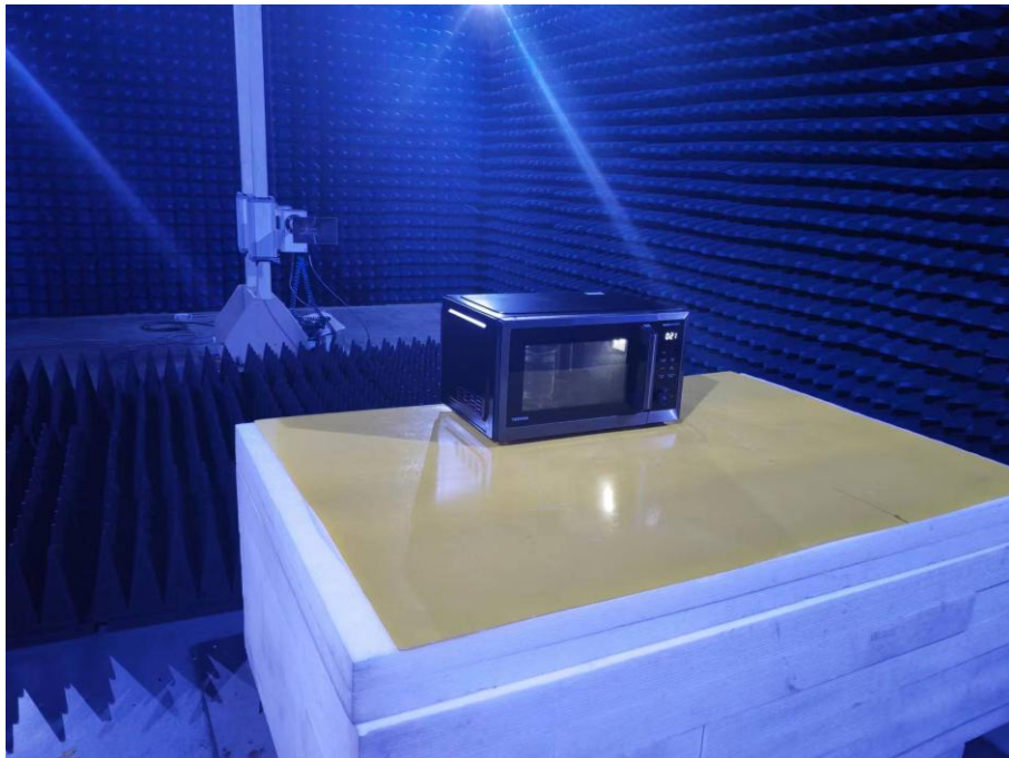
Photo of Radiated Emission Measurement Above 1GHz
